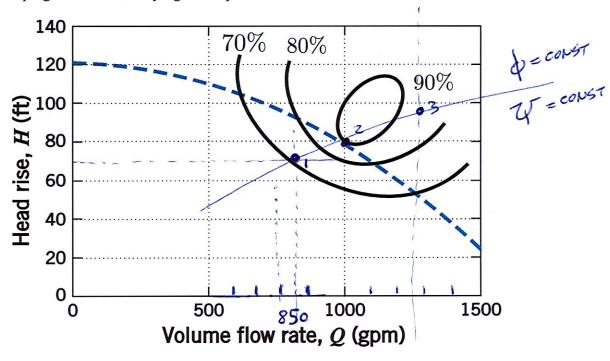
Using the point of max efficiency at  $D = D_2$  as a reference for dimensional scaling,
