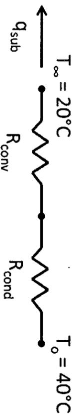
$$R_{conv} = \frac{1}{hA} = \frac{1}{20 \text{ W/m}^2 \cdot \text{K}} = \frac{1}{(20 \text{ W/m}^2 \cdot \text{K})(0.05 \text{ m})^2} = 20 \frac{\text{K}}{\text{W}}$$
