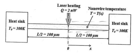
(a) Determine the <u>thermal conductivity of the nanowire</u> if the measured steady-state temperature at the centerline is T(x=0) = 310 K when Q = 2 nW of power are applied to the nanowire. (10 Points)
