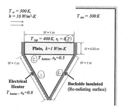
(a) Consider a unit depth of the oven enclosure (i.e., one meter along the direction into the paper) and use the values and symbols provided in the problem. Draw a radiation network for the enclosure of oven's three internal surfaces, and clearly label the resistances, nodal potentials and heat fluxes.
