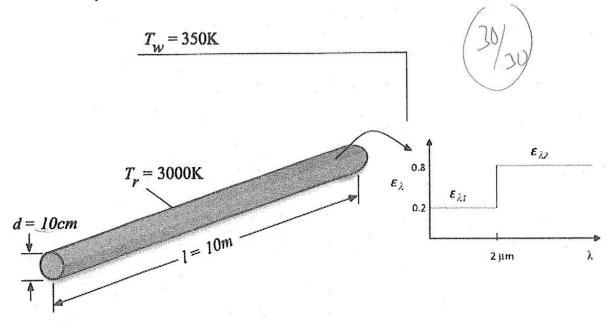
(a) Determine the total emissivity of the fuel rod surface.
