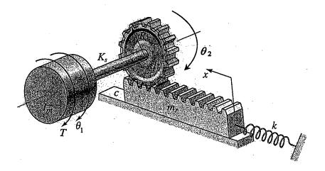
a) Draw free body diagrams for <u>all</u> the elements in this system. Make sure to include all displacements and label all the forces.
