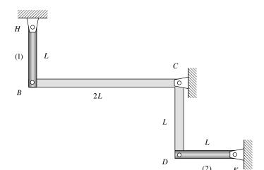
Identical elements (1) and (2) (each having a Young's modulus E, coefficient of thermal expansion  $\alpha$  and cross-sectional area A) are connected between ends B and D, respectively, of a rigid, L-shaped bar BCD. The temperature of (1) is *increased* by an amount of  $\Delta T > 0$ , with the temperature of element (2) being held constant.
