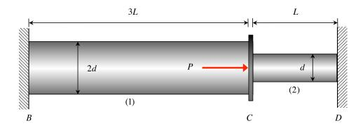
A rod is made up of solid elements (1) and (2) joined by a rigid connector C, with the material of (1) and (2) having the same modulus of elasticity E. An axial load P is applied to C with no thermal loads being present. Let  $F_1$  and  $F_2$  represent the axial loads in elements (1) and (2), respectively. Circle the response below which most accurately describes the relative sizes of  $\left|F_1\right|$  and  $\left|F_2\right|$ :
