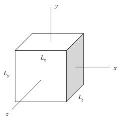
A cube of dimensions  $\left(L_x,L_y,L_z\right)$  experiences a state of stress with uniform components of stress though out the cube. The material of the cube has a Young's modulus of E and a Poisson's ratio of v=0.4. As a result of the loading on the cube, it is known that  $\sigma_y=\sigma_z=\sigma_x/2>0$ . As a result of this loading (circle the correct answer):
