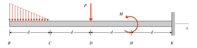
The above loading is applied to a cantilevered beam. *Circle* the figure below which most accurately describes the internal shear force resultant in the beam between locations B and C.
