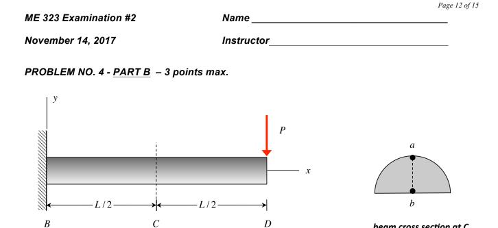
Consider the cantilevered beam above with the concentrated load P at end D. Consider the axial components of stress at points "a" and "b" ( $\sigma_a$  and  $\sigma_b$ , respectively) at location C along the beam. Circle the response below that most accurately describes the relative sizes of the magnitudes of these two stresses:
