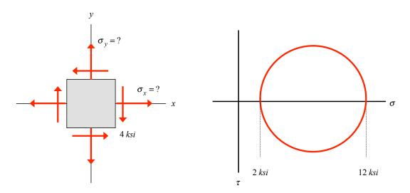
Consider the state of plane stress shown above left where the two normal components of stress,  $\sigma_x$  and  $\sigma_y$ , are unknown. The Mohr's circle for this state of stress is provided in the figure above right. Determine the two normal components of stress  $\sigma_x$  and  $\sigma_y$ . There may be more than one set of answers; you need only find one set.
