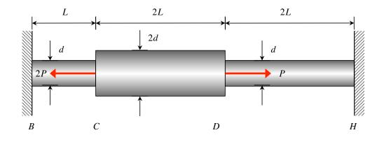
A rod is made up of three circular cross-section components: BC,CD and DH. The material for all components have a Young's modulus of *E*. Suppose you are to develop a finite element model for the rod using one element for each component. If the equilibrium equations after the enforcement of boundary conditions are to be written as:
