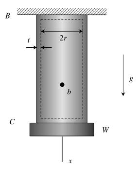
Consider the thin-walled pressure vessel above that contains a gas under a pressure of p. The vessel is attached to a fixed support at B and has a plate of weight W attached to it at end C. Ignore the weight of the vessel. Determine the weight W of the plate for which the *maximum in-plane shear stress* in the vessel at any arbitrary point "b" in the vessel wall is *zero*.
