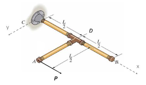
L/2 4/2 P F M, JAP 0 4/2 4/2 A P For member D T. = F + PFisa dummy force. M. = PLZ VZ MZ For member (2) 3 Vz = P $T_2 = 0$ P  $M_2 = PY$  $\mathcal{U} = \mathcal{U}^{O} + \mathcal{U}^{O}$  $\frac{=1(F+P)^{2}L}{2} + \frac{1(FL)^{2}L}{2(Z)EIZ}$ (<sup>1/2</sup> (Py)<sup>2</sup> dy + 142 20/20  $= \underline{L} (F+P)^{2} + \underline{L} (PL)^{2} + \underline{L} P^{2} (L/2)^{3}$   $4EA \qquad 4EE \qquad 4EE \qquad EEL$ = 2 L(F+P) 4EA 200 LP 20EA F=0
