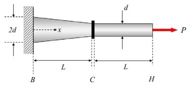
a) Using a **two-element** finite element model (one element per segment), construct the global stiffness matrix. Note that the average cross section area of a "cone frustum", whose ends have circular cross sectional areas  $A_1$ , and  $A_2$ , is given by:
