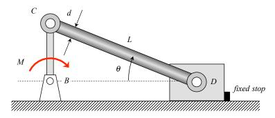
A mechanism is made up on a rigid crank link BC, a connecting rod CD and piston D. CD has a circular cross section with an outer diameter of d and with a length of L. The connecting rod CD is connected to the crank link and the piston with pin joints at C and D. During the operation of the mechanism, under the action of a torque M acting on the crank, the piston is being pressed against a fixed stop, as shown in the figure, keeping the mechanism in equilibrium.
