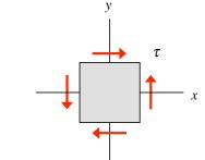
Consider the state of stress shown above in a *ductile* material. Let  $\tau_{MSS}$  and  $\tau_{MDE}$  be the values of the shear stress  $\tau$  above that correspond to failure of the material using the maximum shear stress and maximum distortional energy theories, respectively.
