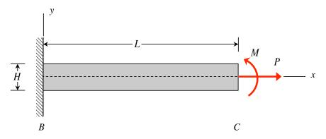
A square cross-sectioned, cantilevered beam has a length of L, a depth of H and is made up of a material with a Young's modulus of E. A bending couple M and an axial load P are applied to end C of the beam. The x-axis runs along the midline of the beam.
