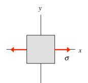
Consider the state of stress shown above in a *ductile* material. Let  $\sigma_{MSS}$  and  $\sigma_{MDE}$  be the values of the normal stress  $\sigma$  above that correspond to failure of the material using the maximum shear stress and maximum distortional energy theories, respectively.
