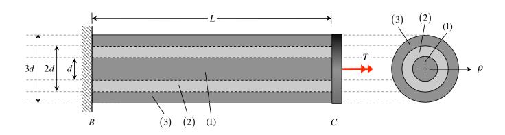
A shaft is made up of three concentrically aligned elements (1), (2) and (3), with these elements having outer diameters of d, 2d and 3d, respectively. The material makeup of these elements have shear moduli of  $G_1 = 3G$ ,  $G_2 = 2G$  and  $G_3 = G$ . All three elements are attached to a rigid wall at end B and to a rigid connector at end C. A torque T acts on the rigid connector at C, as shown in the above figure.
