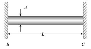
A circular cross-sectioned rod has outer diameter of d, a length of L and is made up of a material with a Young's modulus of E and thermal coefficient of expansion of  $\alpha$ . The rod is attached to rigid walls at ends B and C. With the rod being initially unstressed, the rod is heated in such a way that the temperature of the material in the rod is uniformly raised by an amount of  $\Delta T$ . After this increase in temperature:
