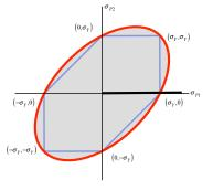
From this, we see that the principal components of stress lie on the  $\sigma_{P1}$  axis. The failure boundary on the  $\sigma_{P1}$  axis corresponds to a location where MSS and MDE results coincide.
