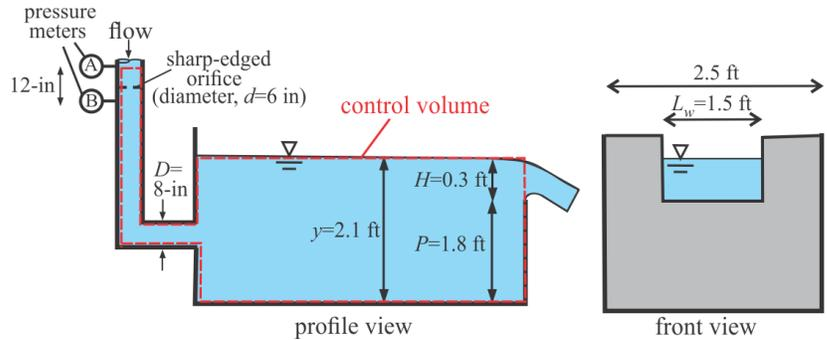
$$Q_{weir} = \underbrace{\left[0.6 + 0.08 \frac{H}{P}\right]}_{C_{d,rw}} \sqrt{2gH^3} = \left[0.6 + 0.08 \left(\frac{0.3 \text{ ft}}{1.8 \text{ ft}}\right)\right] \sqrt{2(32.2 \text{ ft/s}^2)(0.3 \text{ ft})^3} = 0.81 \text{ ft}^3/\text{s},$$
