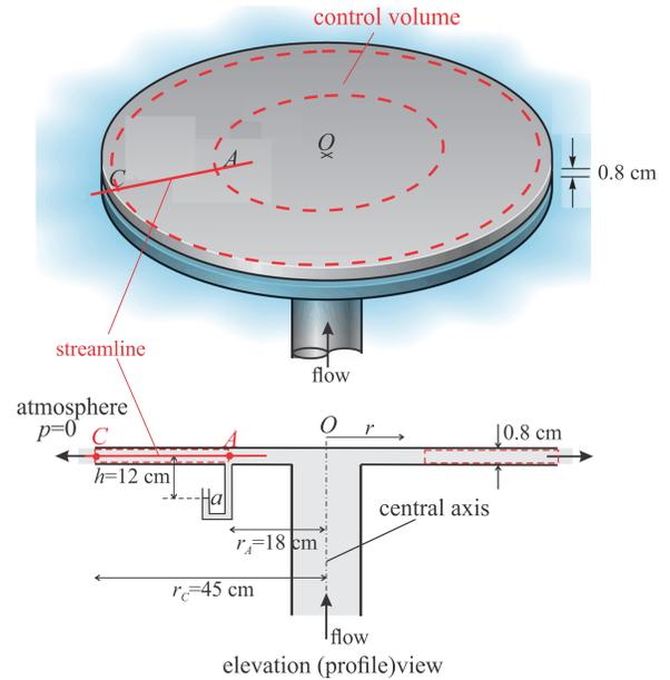
**Solution:** The Bernoulli equation is applied on the streamline shown between the point  $A$  and a point at the exit  $C$  (these points are chosen because information is available at  $A$  and at  $C$ , and information is wanted at  $C$ ):
