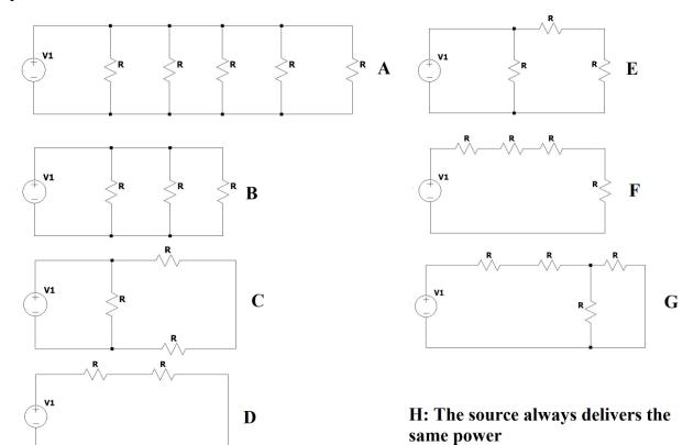
9. If all resistors and sources are the same, in which circuit does the source deliver the least power?
