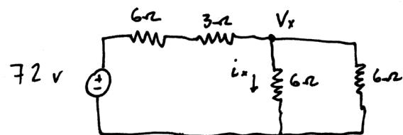
$$V_x = \left( \frac{6 \parallel 16 \Omega}{6 \parallel 16 \Omega + 9 \Omega} \right) (72 V) = \left( \frac{1}{4} \right) (72 V) = 18 V$$
