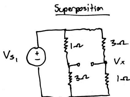
$$\left( \frac{1\Omega}{1\Omega + 3\Omega} \right) (V_{s1}) = V_x \text{ due to } V_{s1}$$
