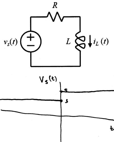
13. What is the value of  $i_L(t)$  in amperes at  $t = 0.6 \text{ s}$ ?
